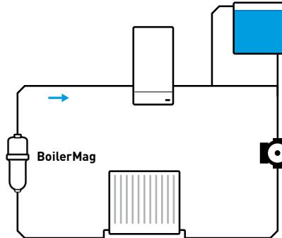
For best results install BoilerMag after the last radiator, prior to the boiler return. Ensure that there is adequate access to the BoilerMag for servicing and maintenance. To prevent frost damage do not install in locations where temperatures can fall below zero°C.
