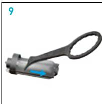
UK Magnetic contamination (black sludge) will be held on the cartridge (8). Using the bowl spanner, slide the contamination deposits to the top of the cartridge (9).
