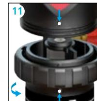
UK Replace the cartridge: the 3 cartridge splines align to the grooves in the bowl wall (10). Check that the 'O' ring is still seated correctly. Hold the bowl to the lid, line up the spigots on each then hand tighten the bowl locking collar (11). **Do not overtighten.**
